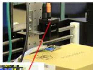
Vision sensor checks orientation of circuit
